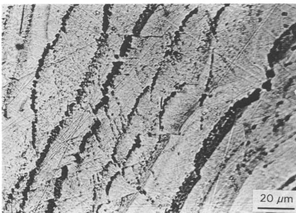
Figure 3 Microstructure of Ag-Zn binary alloy internally oxidized at 800 °C in air.
